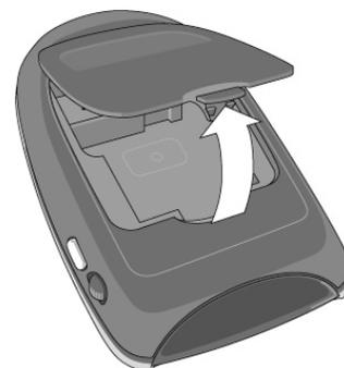
2. Place the battery pack in the battery compartment (refer to illustration on the next page).
