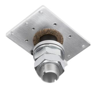
The Crestron® TS-770/1070-SMK is a low-profile swivel mount accessory for TS-770 and TS-1070 series tabletop touch screens. The TS-770/1070-SMK provides a means for permanently mounting the touch screen to a tabletop surface while retaining the ability to rotate it for optimal positioning. The swivel range can be customized using optional limiting screws, with a maximum 330-degree rotation permitted.
