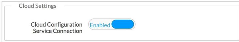
To disable the connection to the cloud server, move the **Cloud Configuration Service Connection** slider to the **Disabled** position. To enable it again, move the slider to **Enabled**.
