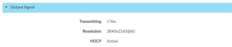
The Output Signal section of the Output page displays read-only information about the output resolution of the device and whether the device is transmitting or not:
