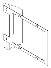
The plate is designed to provide the necessary support for a single touchpanel and can mount to the right or left side of a stud. Confirm that the PMK-3000L is level before application of drywall. A rectangular opening with the dimensions shown in the illustration after this paragraph must be made in the drywall. Verify that the opening exposes the #6-32 tapped holes in each corner.
