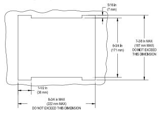
If the opening for the touchpanel in the drywall is too large, two pre-construction accessories are available to make adjustments. Use the optional TMK-3000L (Trim Ring Kit) to provide a smooth edge at the opening. This option provides a finished appearance and is preferred when wallpaper is hung. Use the optional MMK-3000L (Mud Ring Kit) to fill in larger irregularities around the opening (requires plastering).
