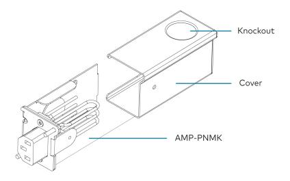
2. Remove the required knockout for AC cable entry. (There are two knockouts, one on the top surface of the plenum kit and the other on the right side. Either can be removed for cable entry.)
