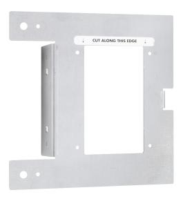
The Crestron® TSW-UMB-570P-PMK preconstruction mounting kit provides a complete preconstruction mounting solution for TSW-570P series portrait touch screens. The TSW-UMB-570P-PMK is designed to be used along with the TSW-UMB-70 universal mounting bracket and permits fastening to the left or right-hand stud of a framed wall prior to installing drywall.
