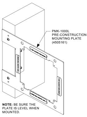
CAUTION: Allow an air gap of at least 12 inches (30.48 cm) in the wall cavity above and below the controller for heat dissipation.
