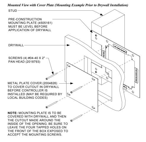
**NOTE:** The four tapped holes on the front of the mounting plate must be exposed to accept the controller mounting screws. These holes are found beneath the drywall just outside the four corners of the opening made by cutting out the drywall. Refer to the **NOTE** in "Mounted View with Cover Plate" illustration above.
