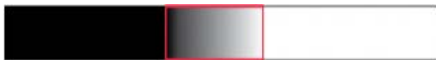
Fig 2: The dynamic range (shown in red) captured with WDR OFF. The area to the left is underexposed, and the area to the right is overexposed.
