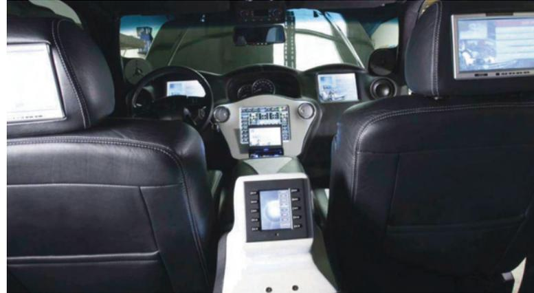
**The Crestron 12" tilt touchpanel forms the dashboard's centerpiece as well as the main controller for the car's controls, lights and AV system. It gives the interior a smooth, uncluttered finish.**
