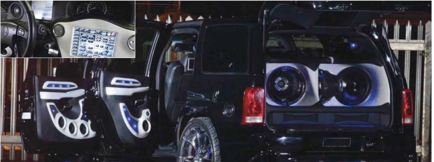
lovingly completed to the very highest standards. No screws show; in fact, some are trimmed in white leather, and some are pieces of grille cloth-finished smoked Perspex (a lightweight plastic), which looks black in the daylight but glows with a blue light that shines through at night. Panels are custom-made, and finished in silver, white, and gray leather. Inside and out, the car features an eye-catching blue glow.
