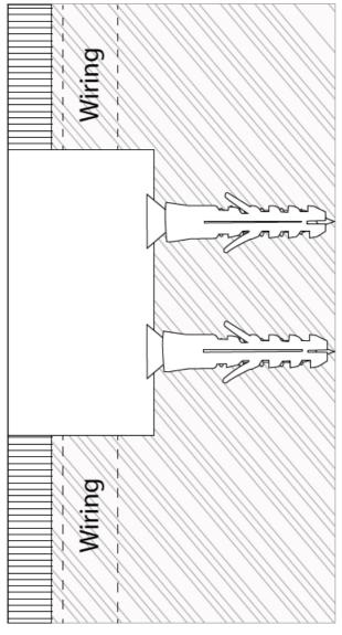
The Edge of the BBI-CBF should be no less than 5mm from the finished wall or surface.
