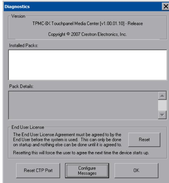
**Reset CTP Port** resets the default value of the CTP port to 41795, for terminal connection using Crestron Toolbox.
