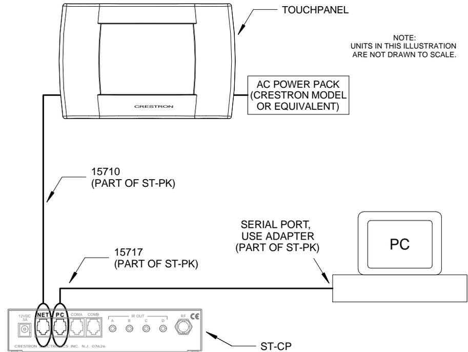
1. Before making any connections to the touchpanel, verify that control system is properly connected to the PC (for ST-CP, use cable 15717 and adapter) and powered on.
