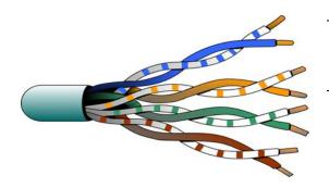
**NOTE:** Do not untwist the two wires in a single pair for more than 1/3-1/2" (0.84 – 1.27 cm) when making a connection. The twists are critical to canceling out interference between the wires.
