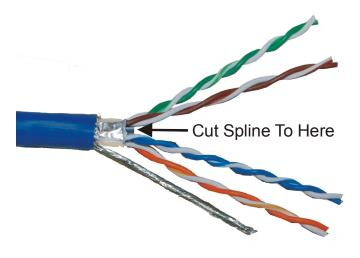
6. Neatly wrap the twisted braid around the foil shield as shown in the following illustration. Only the silver side of foil shield is conductive.
