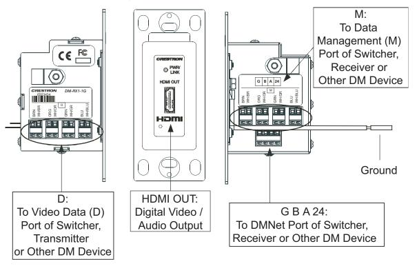
**NOTE:** Ensure the unit is properly grounded by connecting the chassis ground lead to an earth ground (building steel).
