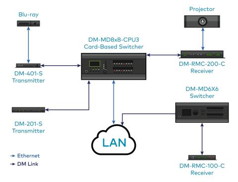
The main Ethernet uplink to a DM system occurs at the DigitalMedia switcher.
