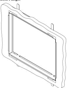
**NOTE:** The mounting plate will have slight play; this is normal. It allows for minor adjustments to the TPS-3100L during installation.
