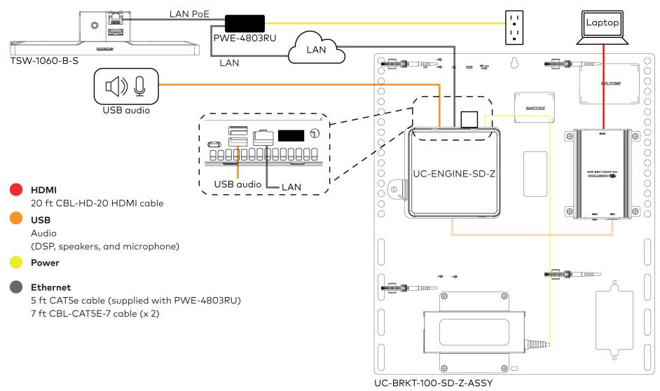
3. Connect the display device and camera to the UC-ENGINE-SD-Z as shown below.
