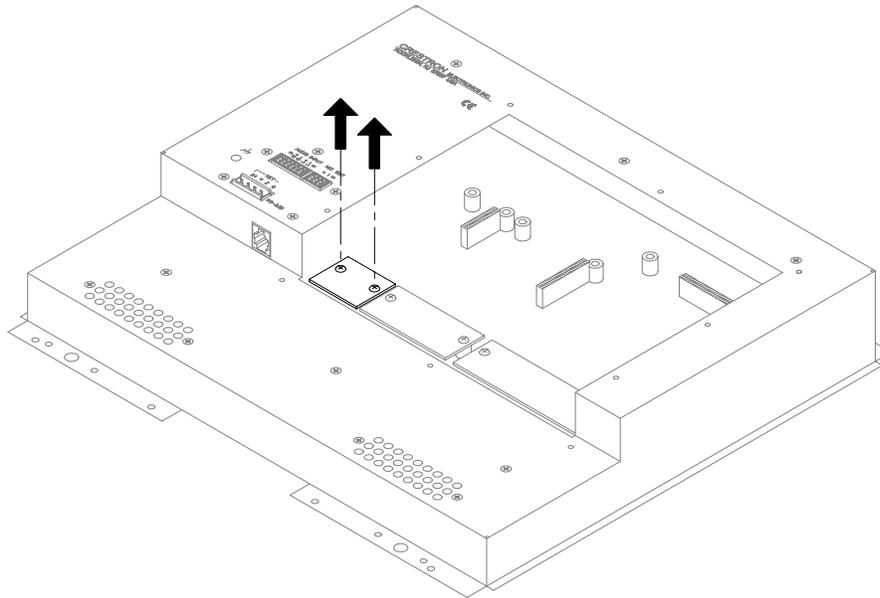
5. As shown on below, align the pins on the touchpanel interface connector of the TPS-ENETL with the touchpanel motherboard connector.
