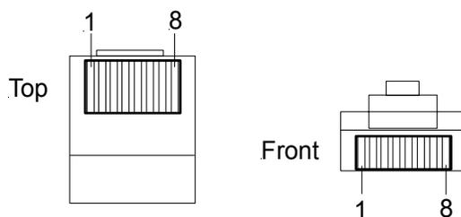
**NOTE:** To determine which is pin 1 on the cable, hold the cable so that the end of the eight pin modular jack is facing away from you, with the clip down and copper side up. Pin 1 is on the far left.
