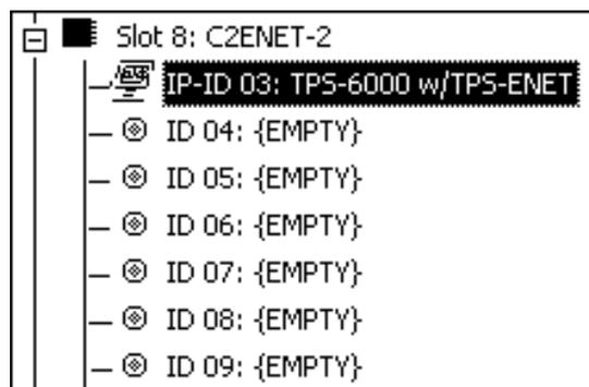
**NOTE:** SIMPL Windows automatically changes the IP ID values of a device added to a program if a duplicate device or a device with the same default IP ID already exists in the program. Always ensure that the network device IP IDs set via Viewport match the ones in your SIMPL Windows program.
