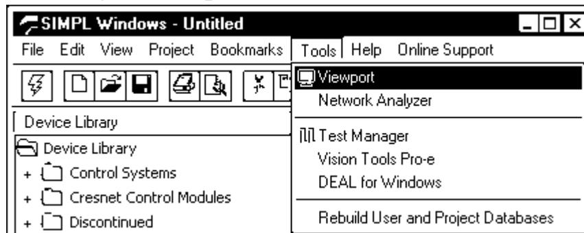
5. Refer to the figure on the next page. While the Viewport is displayed, select **Setup | Communications** (alternatively, depress **Alt+D**) to open the “Port Settings” window.
