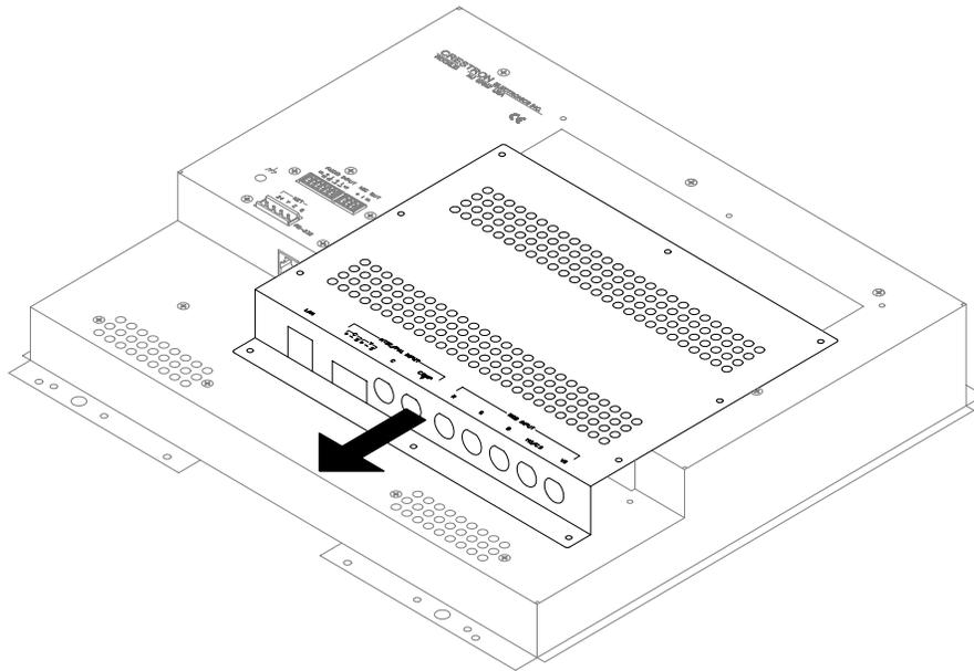
4. Refer to the diagram on next page. Using a #1 Phillips screwdriver, loosen and remove the **two** screws that secure the PCB blank plate and remove the plate.
