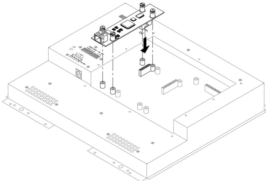
6. **DO NOT** force pins into connector. Press TPS-ENETL until pins are fully seated. Make sure that the mounted screws align with mounting posts of the motherboard.
