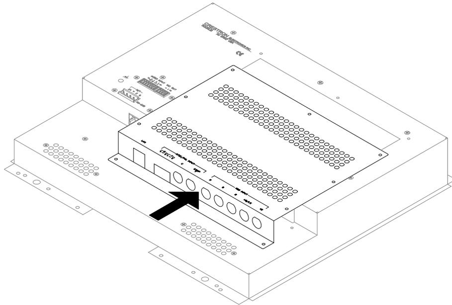
9. Refer to the diagram on next page. Re-install the **10** rear cover screws to **finger-tight** then, using a #1 Philips screwdriver, tighten an additional **1/8-turn**.
