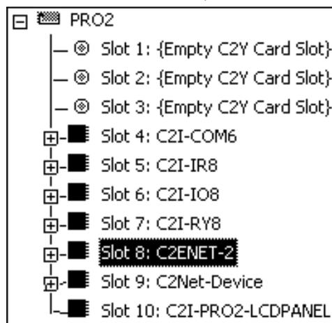
Drag the appropriate Ethernet TPS touchpanel (for example, the TPS-6000 w/TPS-ENET) from the *Touchpanels* folder and drop it on Slot 8 in *System Views*. The lower pane shows the touchpanel in IP-ID 03 (refer to graphic on next page).
