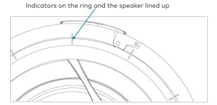
**NOTE:** The lock tab will not lock unless the speaker and bayonet ring indicators fully align.
