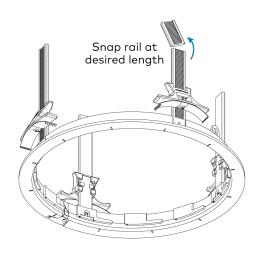
3. Insert the bayonet ring into the hole in the ceiling by bending the rails inward.
