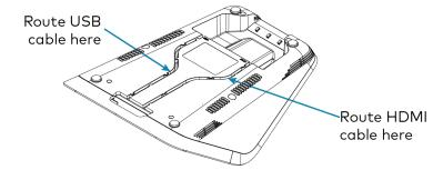
**NOTE:** If the system design dictates that the USB and HDMI Input cables should not exit through the front but at the rear with all other cables, the USB and HDMI input cables should be bundled and secured to the cable retention plate on the underside of the CCS-UC-1-X. Make sure to leave enough cable for a 2- to 3- inch service loop before exiting the rear of the device.
