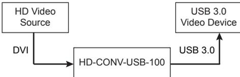
**NOTE:** The HD-CONV-USB-100 can also accept HDMI® video with an appropriate adapter (not supplied).
