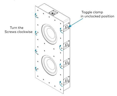
3. To remove the speaker, turn the screws counterclockwise until the toggle clamps rotate inward. Remove the speaker carefully from the hole.
