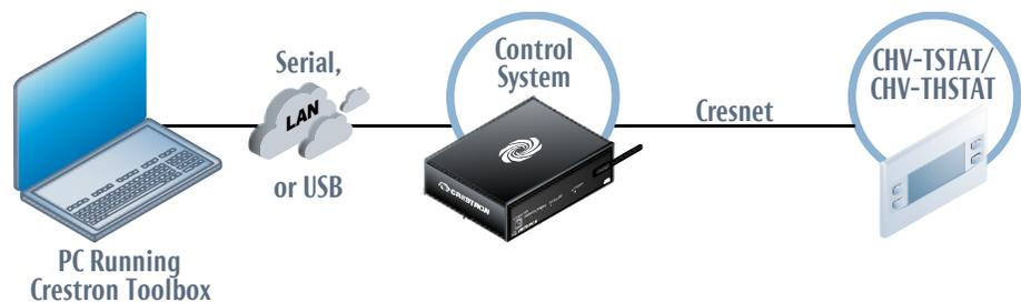
CHV-TSTAT/CHV-THSTAT connects to control system via Cresnet:
