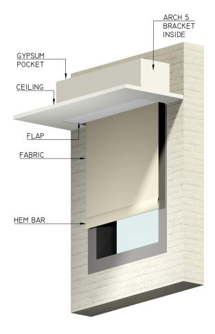
ISOMETRIC VIEW REGULAR ROLL SHADE ABOVE CEILING IN A GYPSUM POCKET WITH POCKET FLAP
