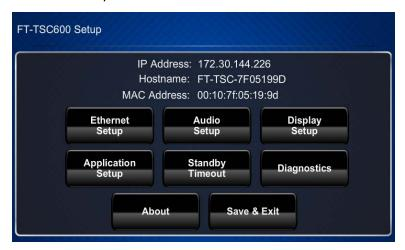
The FT-TSC600 Setup screen is comprised of buttons for Ethernet setup, audio setup, display setup, application setup, standby timeout, and diagnostics. In addition, there is an **About** button that provides information about the touch screen and a **Save & Exit** button. The functions of each are detailed in the following pages of this guide.
