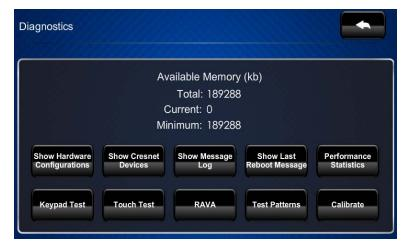
The **Diagnostics** screen displays the available memory and contains controls to show hardware configurations, show Cresnet® devices (to display all devices on the Cresnet network), show the message log, show the last reboot message, and show performance statistics. In addition, there are controls to open various test screens and to initiate touch screen calibration. These are explained in the sections that follow.
