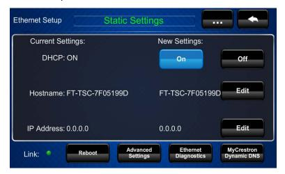
The **Ethernet Setup** screen displays current settings, such as whether DHCP is on or off, the touch screen's hostname, and its IP address. This screen also contains a link indicator to show the status of the Ethernet connection. Controls on this screen are explained in the sections that follow.
