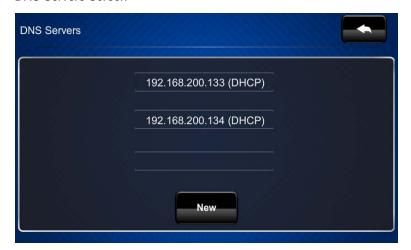
The **DNS Servers** screen provides controls for adding or deleting the IP addresses of DNS (Domain Name System) registered computers on the network. To add a server's IP address, tap **New** to open an on-screen keyboard.
