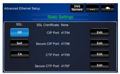
The **Advanced Ethernet Setup** screen provides controls for enabling or disabling SSL (Secure Sockets Layer) and for editing the CIP port, secure CIP port, CTP port, and secure CTP port.
