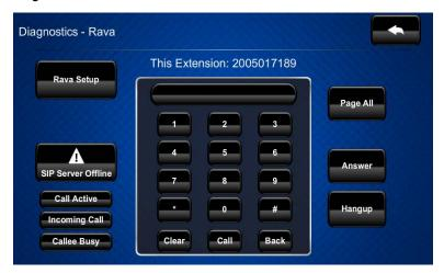
The **Diagnostics - Rava** screen provides controls for testing the use of Crestron's Rava<sup>®</sup> SIP Intercom with the FT-TSC600. It can be used to test projects and settings. If the intercom works but the project does not, there is an issue with the project; if the intercom does not work, there is an issue with the settings.
