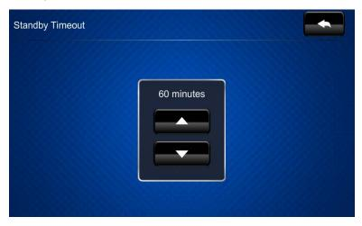
The **Standby Timeout** screen provides controls to adjust standby timeout from 0 to 120 minutes.
