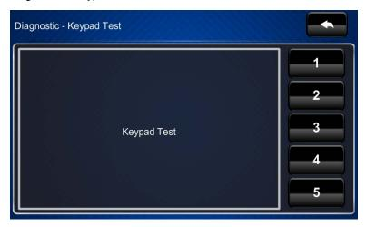
The **Diagnostic – Keypad Test** screen can be used to test the function of the hard keys. When a hard key is pressed, its corresponding indicator on the screen lights.
