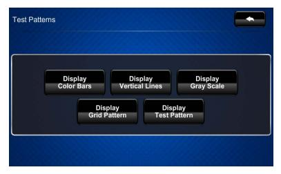
The **Test Patterns** screen contains buttons for selecting the different available test patterns: Display Color Bars, Display Vertical Lines, Display Gray Scale, Display Grid Pattern, and Display Test Pattern.
