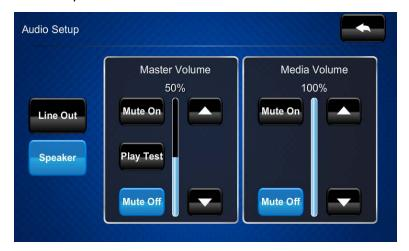
The **Audio Setup** screen provides controls for muting or unmuting the audio, adjusting levels for both the master volume and the media volume, and playing a test .wav file. The **Media Volume** controls adjust the H.264 streaming media level in relation to the **Master Volume** controls. Use the **Line Out** and **Speaker** buttons to choose whether audio plays via the line output or through the internal speaker.
