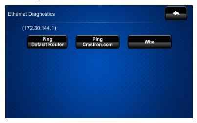
The Ethernet Diagnostics screen provides controls for verifying connections. Tap Ping Default Router to verify connection to the router. (The screen displays a "Passed" message to show successful connection.) Tap Ping Crestron.com to verify connection to an external DNS server.
