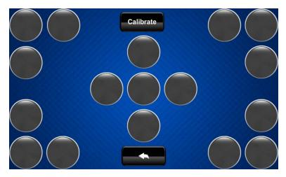
The touch test screen can be used to test the function of the screen. When a location button is tapped, its indicator on the screen lights. This screen also contains a **Calibrate** button to initiate touch screen calibration.
