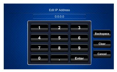
Use the keyboard to enter the new IP address. Tap **Clear** to remove a previous entry, **Backspace** to delete the last digit, **Enter** to save a new entry, or **Cancel** to return to the previous screen.
