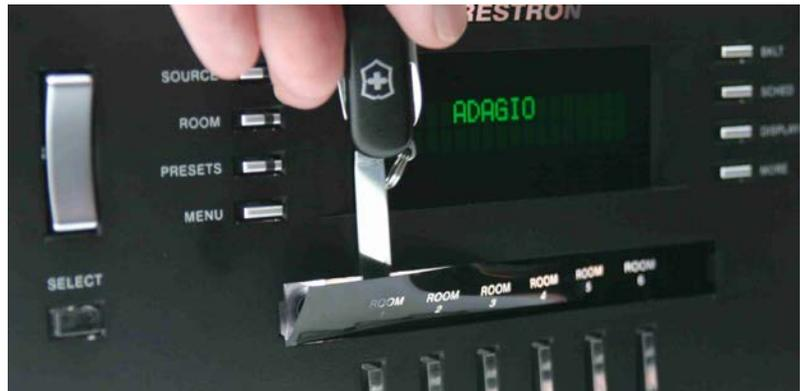
4. Continue sliding the screwdriver until the entire top of the label strip is visible. Remove the label strip by pulling the top of the label strip up from the Adagio component as shown below.
