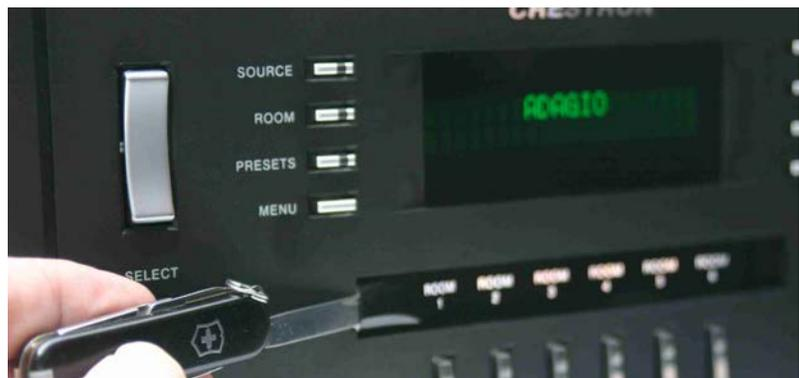
3. Continue sliding the screwdriver behind the label strip until the top of the label strip slides out as shown in the following picture.
