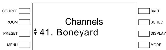
⇒ Press the selection control up or down to browse the list of channels. When the desired channel is displayed, press **SELECT** to select the channel. The display will indicate that the channel has been selected.
