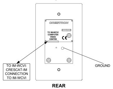
**NOTE:** For optimum performance, Crestron strongly recommends using CRESCAT-IM cable, available from Crestron. Other high-quality/low skew CAT5e/CAT6 wiring may also be used with varying performance. The maximum cable length between the IM-WCVP and the IM-WCVI is 40 feet.
