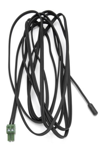
The PC-TS is a remote temperature sensor designed for use with the Crestron® PC-350V series power controllers. The PC-TS monitors the ambient temperature within the equipment rack or room and sends alert notifications if the temperature exceeds the threshold values set in the connected power controller.
