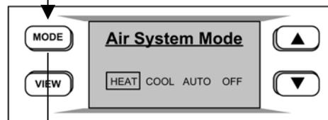
Displays Air System Mode control. Press **MODE** button to continue to Slab System Mode screen.
