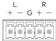
Refer to the following table and diagram for analog audio output pin assignments and connection information.
