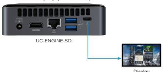
Connect the CBL-USBC-HD-9 to the USB-C port on the UC-ENGINE-SD and to the display..
