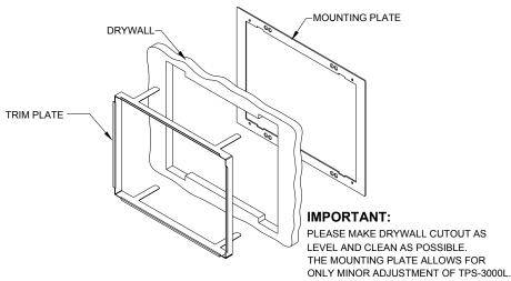
5. Carefully pass the mounting plate through the opening and rest it against the interior surface of the drywall.
