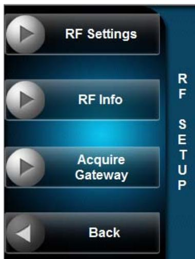
The “RF Setup” menu is divided into three sections: *RF Settings*, *RF Info* and *Acquire Gateway*.
