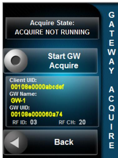
Before the UFO-WPR-3ER can be used, it must be acquired by a CEN-ERFGW-POE Extended Range RF Wireless Gateway.
