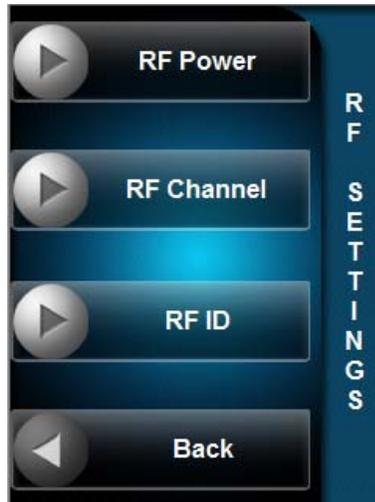
The “RF Settings” menu is divided into three sections: *RF Power*, *RF Channel* and *RF ID*.
