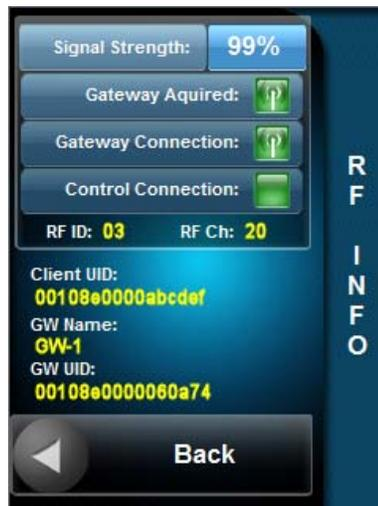
The “RF Info” screen displays RF signal strength, RF ID, RF channel, client UID, gateway name and gateway UID, in addition to providing indicators for when the gateway is acquired, when the gateway is connected and when a control system is connected.
