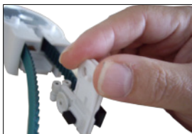
Place Master Carrier on Belt
