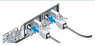
8. Secure the power cable(s) to avoid tangled wires and possible disconnection.
