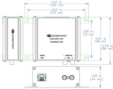
Dimenions typical of any model transmitter or receiver
