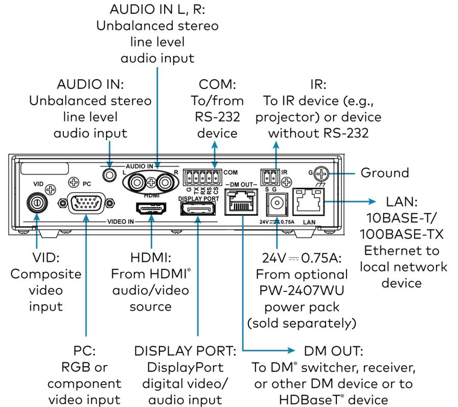
**NOTE:** The DM OUT port is a PoDM (Power of DM) or HDBaseT® PoE (Power over Ethernet) PD (Powered Device) port. To receive PoDM or HDBaseT PoE, the DM-TX-401-C requires a connection to a DM® switcher or other equipment that has a PoDM or HDBaseT PoE PSE (Power Sourcing Equipment) port. Any wiring connected to a PoDM or HDBaseT PoE PSE port is for intrabuilding use only and should not be connected to a line that runs outside of the building in which the PSE is located.
