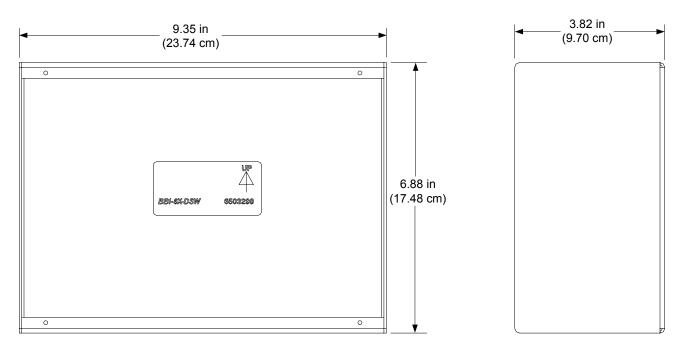
**NOTE:** Knockout holes are intended for Class 2 wiring only and are 1 1/8" (29 mm) diameter.
