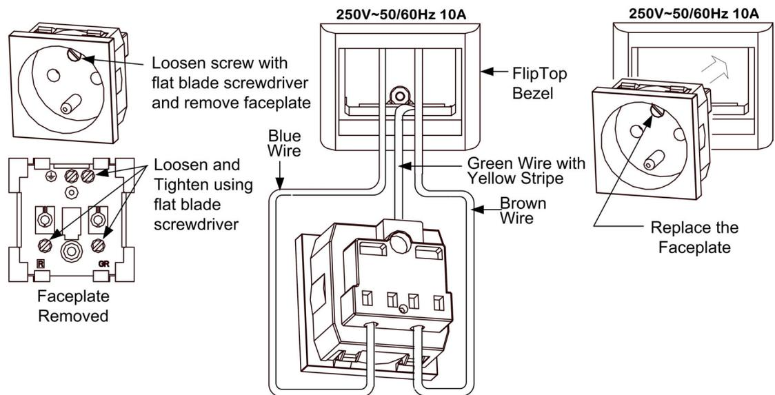
After connecting the wires as shown in the illustration, replace the faceplate, orient the receptacle as shown and snap the receptacle into the bezel.
