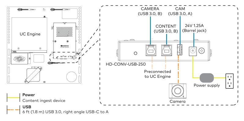
3. Connect power and the content ingest device (HD-CONV-USB-250) to the top of the UC Presentation Transmitter. Connect the UC Engine or LAN to make a direct or network connection as described in step 1.
