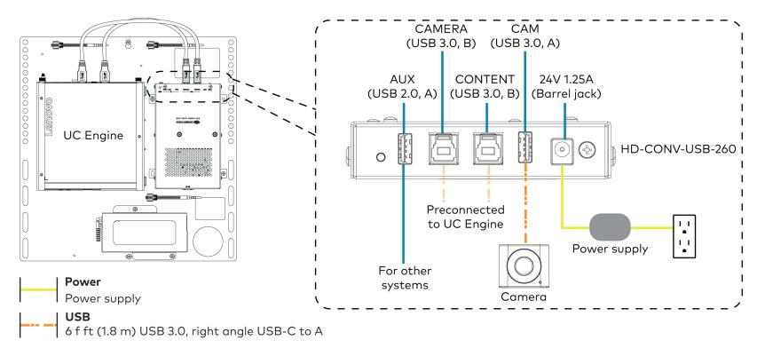
5. Connect power and the content ingest device (HD-CONV-USB-260) to the top of the UC Presentation Transmitter. Connect the UC Engine or LAN to make a direct or network connection as described in step 1.
