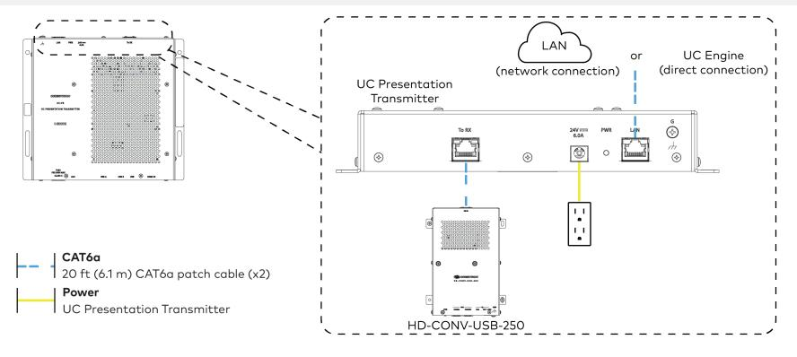
4. Connect the conference device using the included PoE+ injector and USB A to Micro-B cable to the bottom of the UC Presentation Transmitter.
