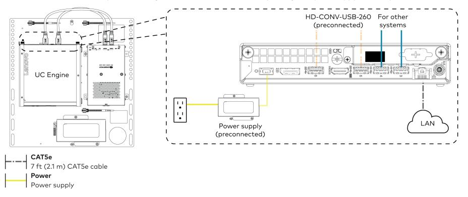
3. Connect displays to the UC Engine.
