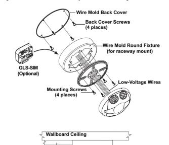
Wire Mold Raceway
