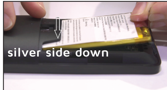
Inserting the Battery into the TSR-310
