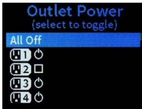
The **Outlet Power** screen is used to power the PC-300 rear outlets on or off.
