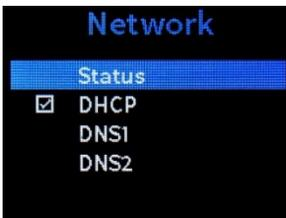
The **Network** screen provides selections to configure general network settings and DNS server settings. This screen also provides a selection for viewing the network status.
