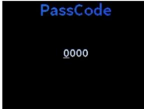
Use the **PassCode** screen to create a new four-digit passcode for accessing the LCD display setup screens.
