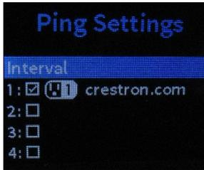
Use the following settings to configure ping monitoring for the PC-300.
