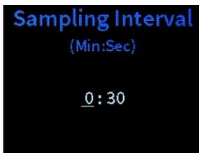
Use the **Sampling Interval** screen to set the sampling interval between event log recordings.
