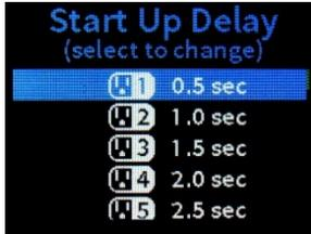
The **Start Up Delay** screen is used to adjust the start up delay time for the rear outlets. After the PC-300 is powered on, the rear outlets power on after their start up delay times elapse.
