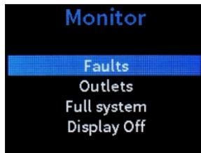
Use the **Monitor** screen to monitor device faults, outlet data, and system sensor readings. The LCD display may also be turned on or off by selecting **Display On/Off**.
