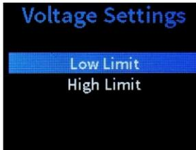
The **Voltage Settings** screen provides selections for setting the under voltage (**Low Limit**) and over voltage (**High Limit**) cutoff limits in volts for the PC-300. The PC-300 shuts off power to the ac outputs when the ac input is detected to have gone over or under the set values.
