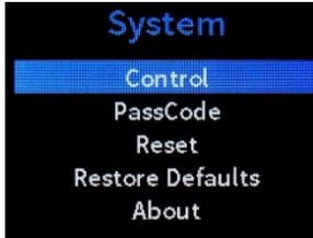
The **System** screen provides selections for configuring the system settings. The **System** screen also may be used to set a new passcode, to reset the PC-300, to restore all settings to their default factory values, and to view device information.
