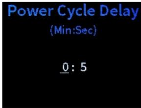
Use the **Power Cycle Delay** screen to set the duration that power to an outlet cycles off before powering back on.
