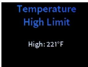
Use the **Temperature High Limit** to set a temperature cutoff limit in the selected temperature unit. The PC-300 shuts off if the temperature is detected to have gone over this value.
