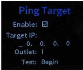
Use the **Ping Target** screen to configure the ping monitoring settings for the selected outlet.
