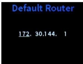
Use the **Default Gateway** screen to enter an IP address for the gateway router that connects the PC-300 to the network.
