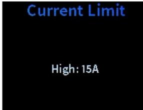
Use the **Current Limit** screen to set the current limits in amperes for the PC-300. The PC-300 shuts off if the combined amperes of the ac outputs are detected to have gone over this value.
