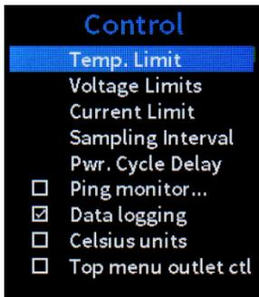
The **Control** screen provides selections for configuring various system settings, including device limits, event log intervals, power cycle delay, ping monitoring, data logging, and LCD display outlet control.
