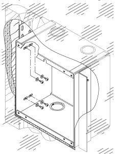
14. As shown below, use a ruler to adjust the back box to approximately 1/16-inch (0.15 cm) *inward* of the face of the gypsum board to accommodate the distance between the back box and the front panel. Using a #2 Phillips screwdriver, tighten the four pair of bracket screws finger-tight plus an additional 1/8-turn.
