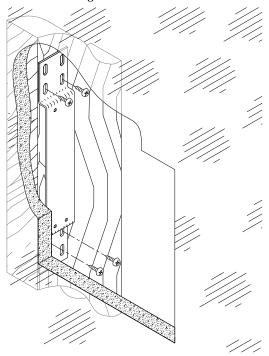
9. Orient the back box enclosure as shown below (notch for manual unlatching **upwards**) and remove an appropriate knockout for the Cresnet wiring.
