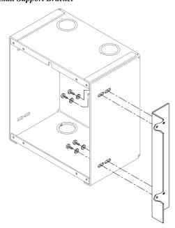
11. Position the back box enclosure near the cut-out area and feed the Cresnet wiring through the enclosure knockout.
