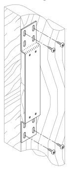
3. Orient the back box enclosure as shown below (notch for manual unlatching **upwards**) and remove an appropriate knockout for the Cresnet wiring.
