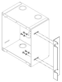
5. As shown below, loosely install **four** pan head screws with washers through the inside of the enclosure into the mounting bracket holes. Tighten screws only **finger-tight** so that final adjustments may be made during step 7 of this procedure.
