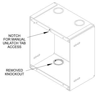
4. As shown below, loosely install **four** pan head screws with washers through the inside of the enclosure into the support bracket holes. Tighten screws only **finger-tight** so that final adjustments may be made during step 7 of this procedure.
