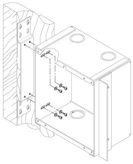
6. Feed the Cresnet wiring through the enclosure knockout.
