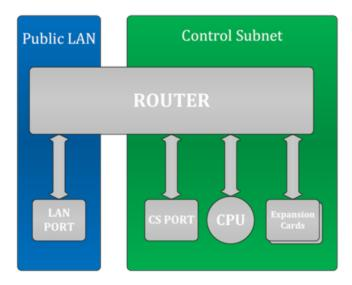
The firewall rules permit entry to only the traffic that is listened to by the CPU. As a result, a port scan will only show ports that are listened to by the CPU. Users can set up manual port forwarding rules to make custom connections to the devices on the Control Subnet.
