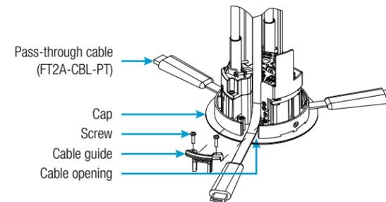
3. Connect the power pack cable and either the USB or Cresnet cable to the connectors located on the underside of the cap. Refer to "DO Connect the Device" for details about each connection.
