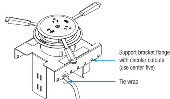
4. Ensure that the loop provides enough cable for the end user.
