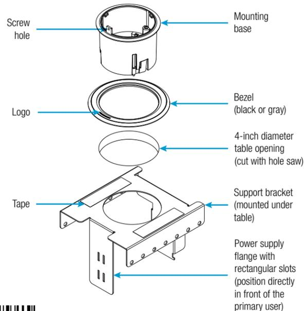
4. Secure the assembled items (mounting base, bezel, and support bracket) to the table.
