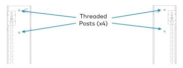
3. Attach the soundbar bracket arms to the threaded posts on the display mounting bracket arms with the nuts and washers removed in step 2.
