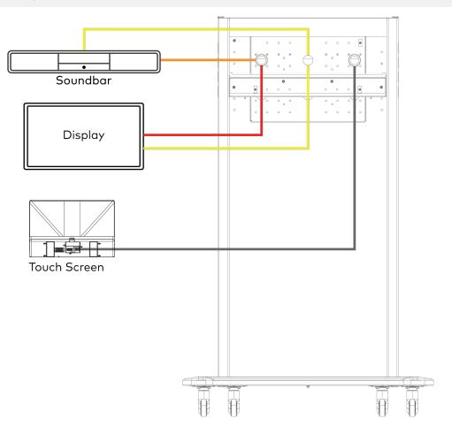
2. Make LAN and power connections from the bottom rear of the cart as shown below using the integrated retractable cables.
