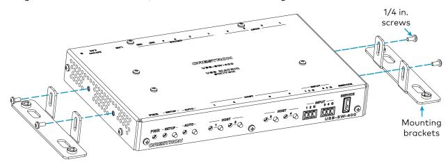
2. Using the included washers, anchors, and 3/4 in. screws, mount the device to a flat surface.
