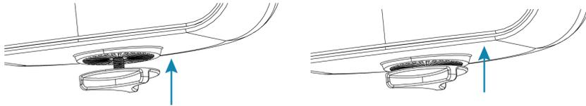
b. Slide the threaded portion of the knobs into the slots in the yoke bracket.
