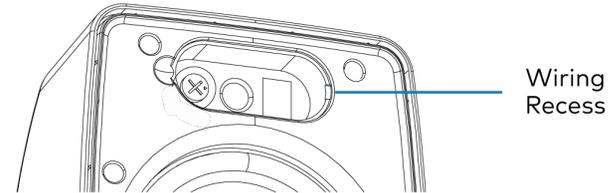
2. Feed the speaker wire slack at the mounting bracket through the wire opening in the speaker. Optionally, thread the speaker wire through the included grommet plug and insert the grommet plug into the wire opening at the rear of the speaker enclosure for additional weatherproofing.
