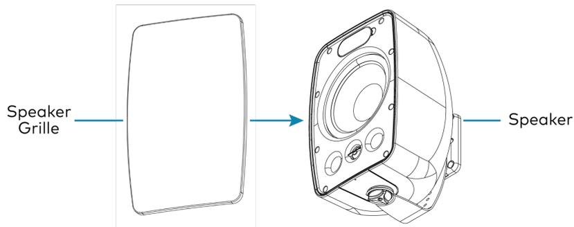
6. Fasten the grille to the top and bottom of the speaker housing using the two security screws removed during step 5a.
