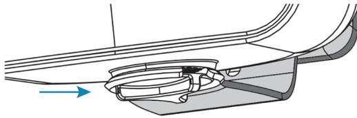
c. Tighten the knobs at the top and bottom to secure the speaker on the yoke bracket at the desired horizontal angle.
