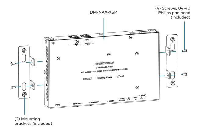
• If mounting the device under a table, orient the mounting brackets to be flush with the top face of the DM-NAX-XSP.
